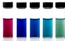
Figure 23.4: Different color fluids containing nano-particles can be obtained by changing the permittivity of the background fluids (courtesy of nanocomposix.com).
